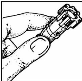
Figure 071-311-2025-26. Holding the extractor pin in
