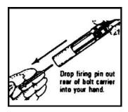
Figure 071-311-2025-14. Removing the firing pin
