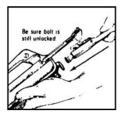
Figure 071-311-2025-33. Placing the bolt carrier
