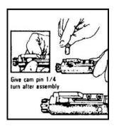
Figure 071-311-2025-28. Replacing the bolt cam pin
