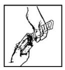
Figure 071-311-2025-42. Removing the magazine spring and the follower
